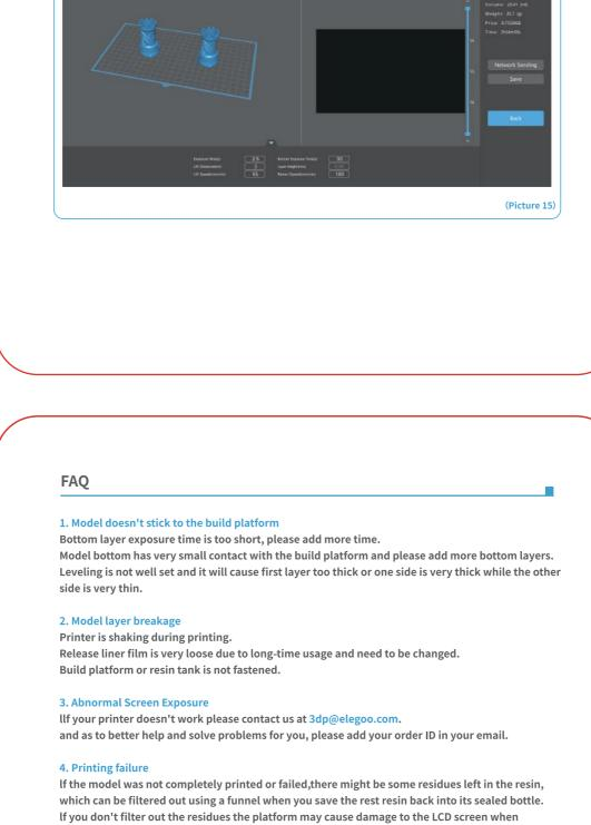
As to the residual resin on the platform and tank, you can clean and wipe them up using tissues.
