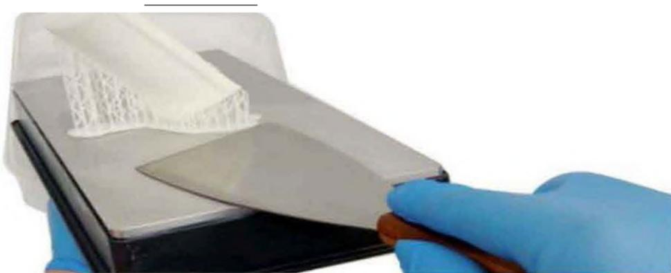
After removal, the model should be cleaned in minimum of ٩٥% alcohol for several minutes, time depends on the model's complexity and size.
