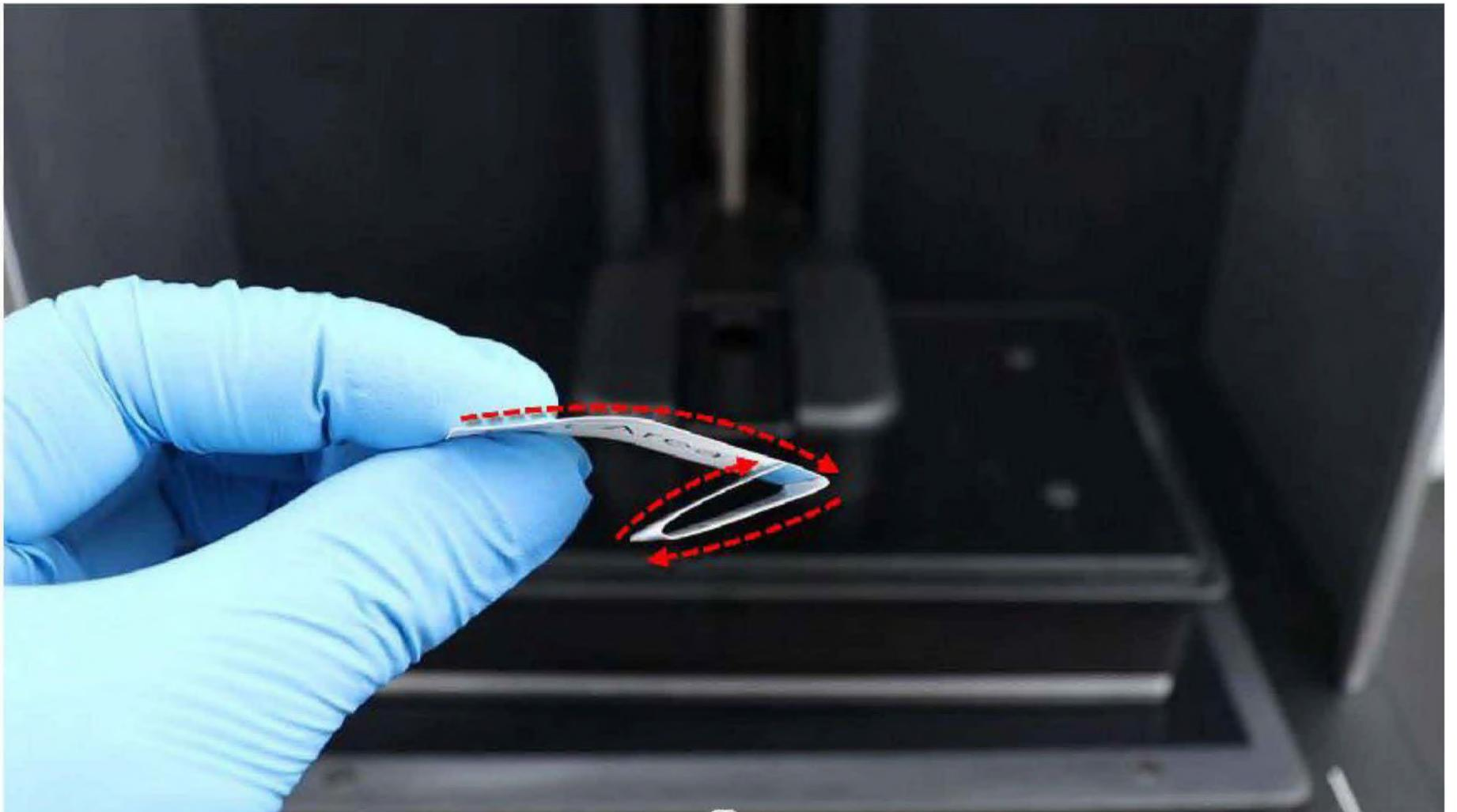
2,3,1) Using the menu on the printer touch screen, select the "Function" icon, "Z-axis Movement", then select the "Z 0" icon. The build plate will descend to the button and press down on the paper strips and leveling paper.
